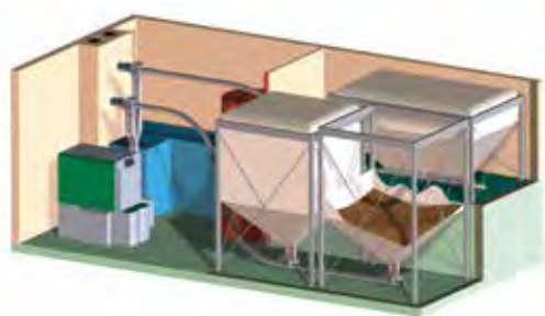
2 Flexilo MAXI and 1 Flexilo TROUGH as feed of 180 kW pellet boiler
